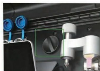
Desiccant replacement window
