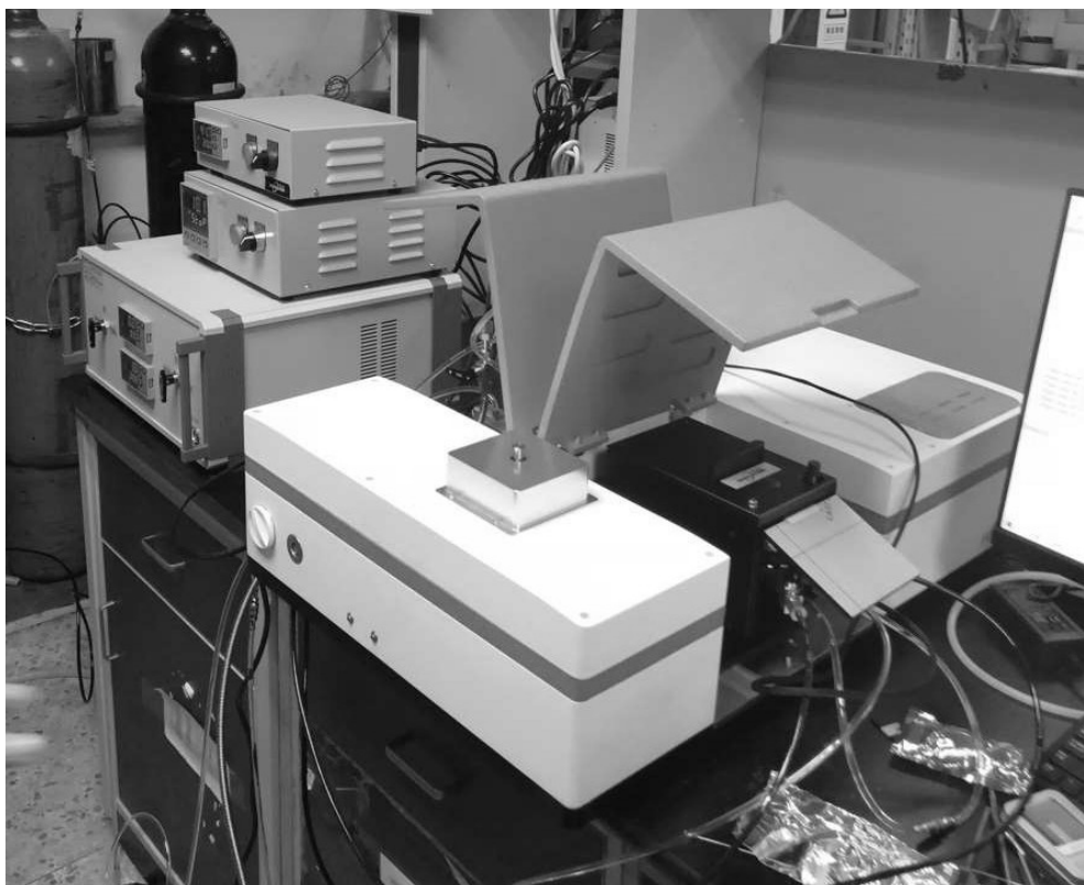
In-situ diffuse reflectance and in-situ transmission on different catalysts at a research institute.
