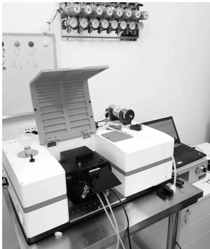
An FI-RXF100-R with an in-situ diffuse reflectance cell, cooling-water circulation and a high-precision temperature controller, in a university laboratory.
