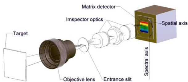
Principle of hyperspectral imaging and basic optical layout
