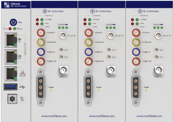
Figure.1 Closed- loop scanner controller - MC-ArchimedesLT.03.Ultra.
