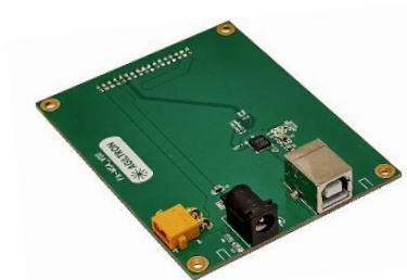
USB/GUI Adopting PCB mounted on top of the component for convenience
