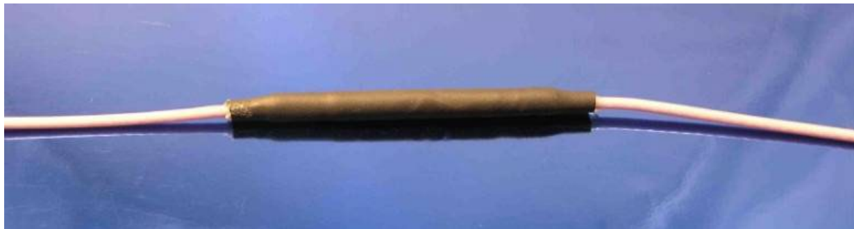
Figure 7. A finished splice (with shrink tube)
