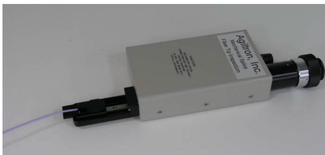
Push down gently to cleave. The cleaver will open when you release pressure.
