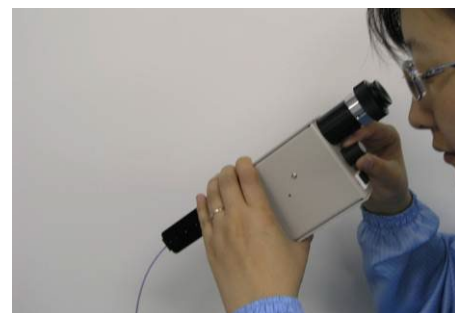
Push down gently to cleave. The cleaver will open when you release pressure.
