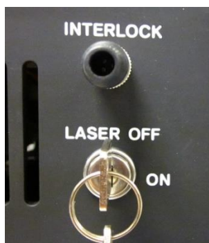
Figure 3.3 Interlock & Ignition Switch
