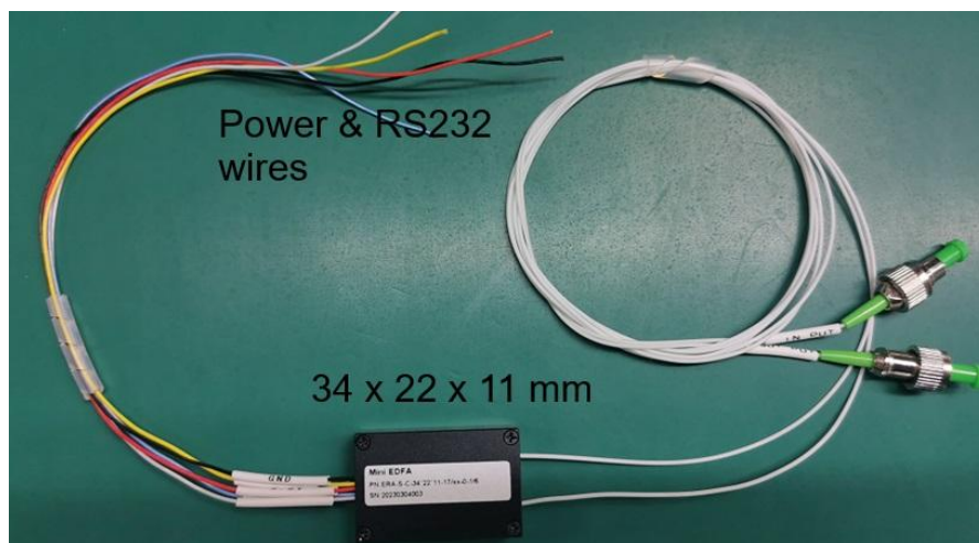
Figure 1 Ports of EDFA
