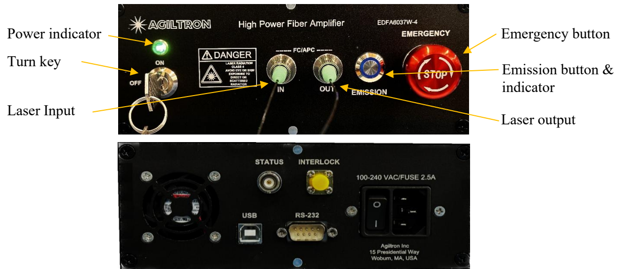
Figure 1: Front and rear panels of EDFA
