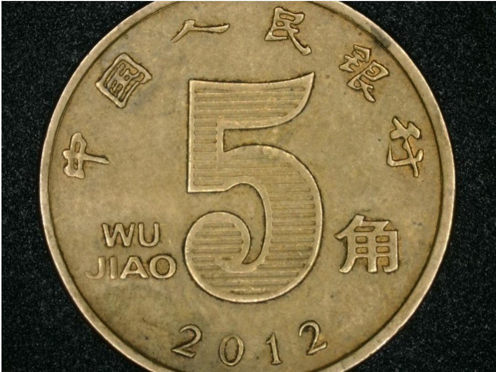
Figure 18 Coin taken under annular light illumination with ZM0480H1080PA
