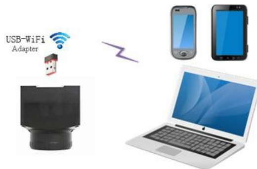
Figure 13 The PC or mobile device connect to the camera through WiFi
