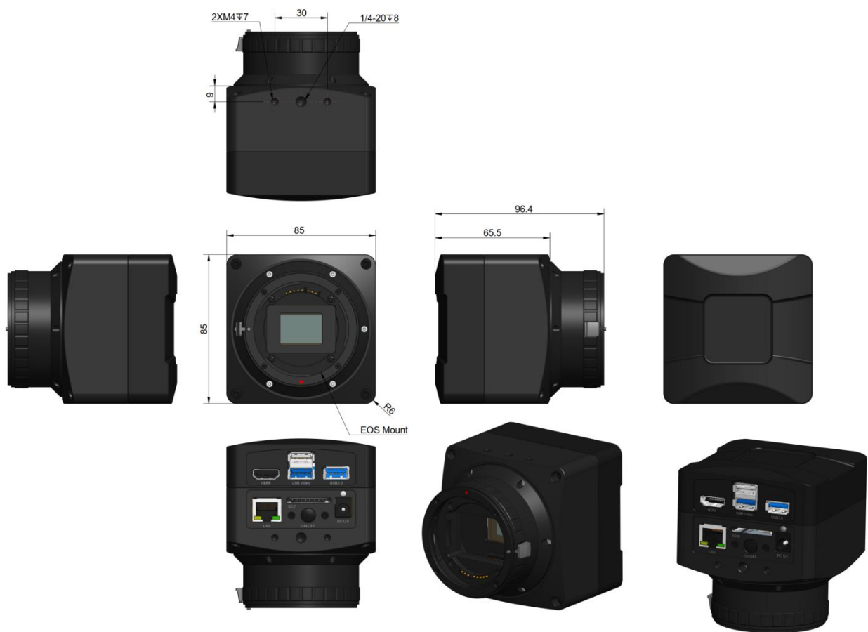
Figure 8 Dimension of X8FCAM4K22MPA_EFL camera
