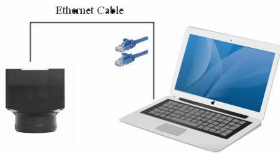
Figure 15 Connecting the X8FCAM4K22MPA_EFL camera with ethernet cable to the PC
