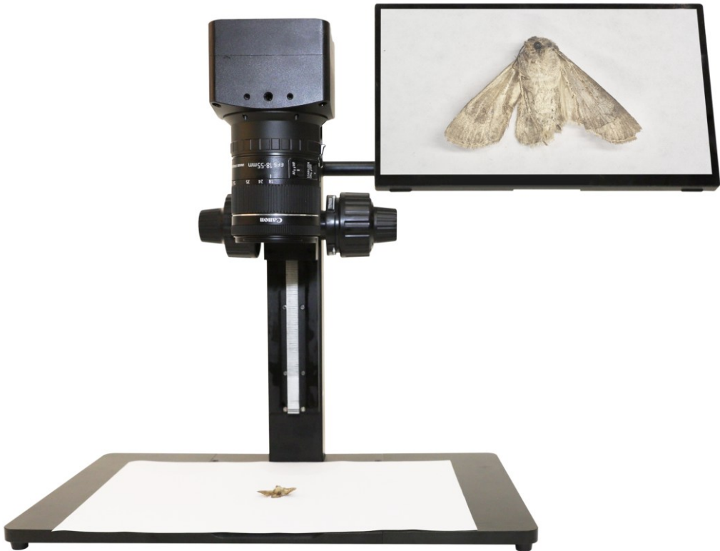
Figure 4-16 TPS-600 bracket+X7FCAM4K16MPA_EFL+Canon EF-S 18-55mm f/4-5.6 IS STM+HDMI 4K monitor
