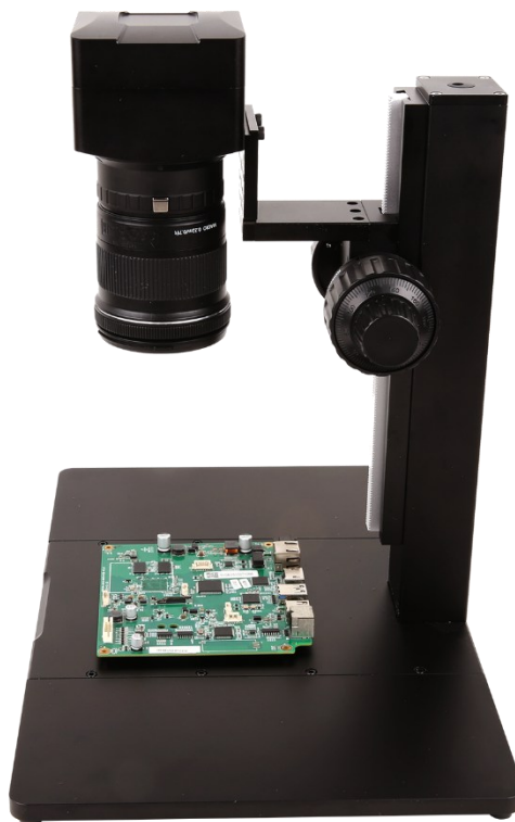
Figure 4-4 TPS-600 bracket+X8FCAM4K22MPA_EFL+Canon EF-S 18-55mm f/4-5.6 IS STM
