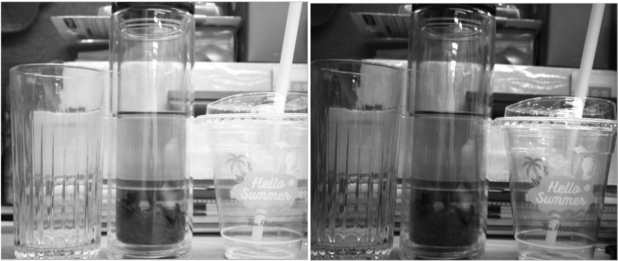
Figure 5-70 Comparison of plastic surface effects between ordinary camera (left) and polarizing camera (right)
