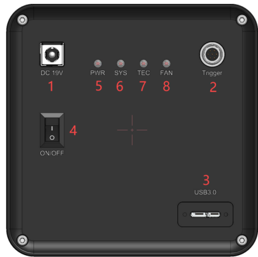
Figure 12-6 MAX251& MAX151&MAX102 Camera interface diagram
