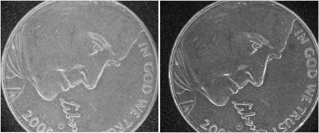
Figure 5-72 Ordinary camera (left) compared with polarizing camera (right) metal surface effect
